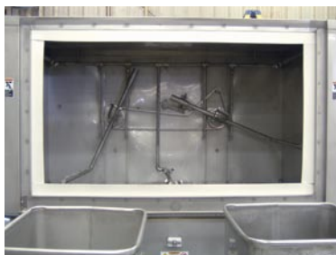
Synchronized rotating spray arms clean inside, outside & bottom of vats.
