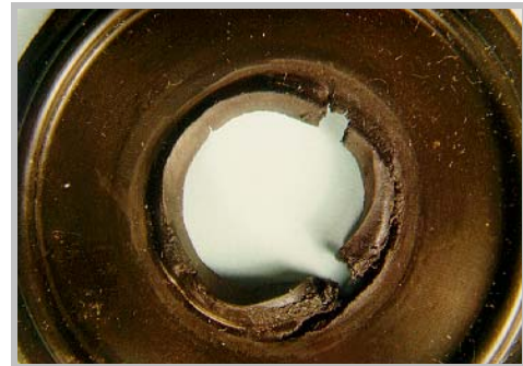
Standard 1" Viton gasket used in a water for injection system after being subjected to multiple steam cycles
